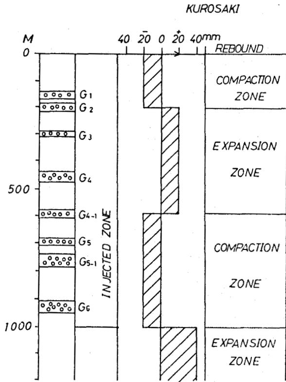
Figure 9.7.13 Columnar section showing the position of expansion and compaction layers at Kurosaiki.
