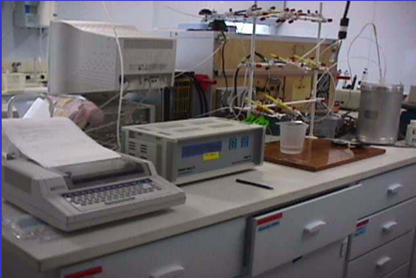
Figure 15. Photograph showing mercury analysis by cold-vapor atomic fluorescence spectroscopy (CVAFS).
