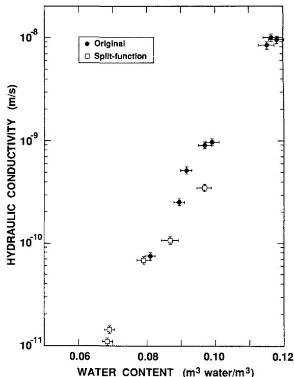
Fig. 4. Hydraulic conductivity vs. water content for Delhi soil, measured with original and split-function reservoir systems.
