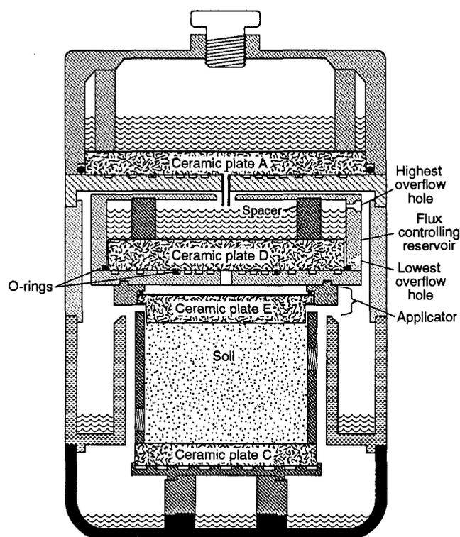
Fig. 2. Apparatus incorporating the split-function reservoir system. The applicator and flux-controlling reservoir replace the constant-head reservoir in Fig. 1.
