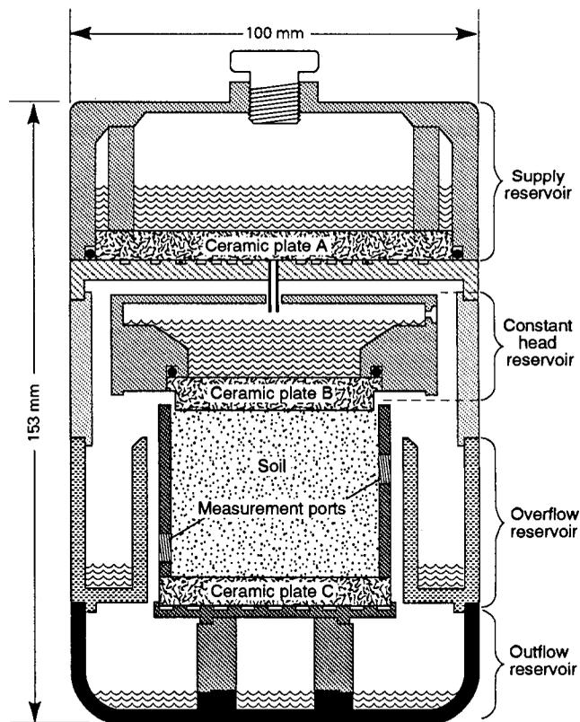
**Fig. 1.** Apparatus essentially equivalent to the original design of Nimmo et al. (1987) for measuring unsaturated hydraulic conductivity by the steady-state centrifuge method. The apparatus fits into a 1-L centrifuge bucket. Materials used for the nonporous components include stainless steel for the soil retainer, acrylic plastic for the supply reservoir, and aluminum for most other parts.
