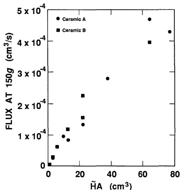
Fig. 3. Comparison of flux with the  $\bar{H}A$  factor, the product of the corrected height factor,  $\bar{H}$ , and the area,  $A$ , of the ceramic through which water flows in the flux-controlling reservoir. Measurements were made with 500-kPa ceramic limiting the flow. Most of these measurements were made at an angular speed of 105.1 s. For graphing, results of the others were converted to their equivalent at 105.1 s by multiplying by the ratio of the centrifugal forces.
