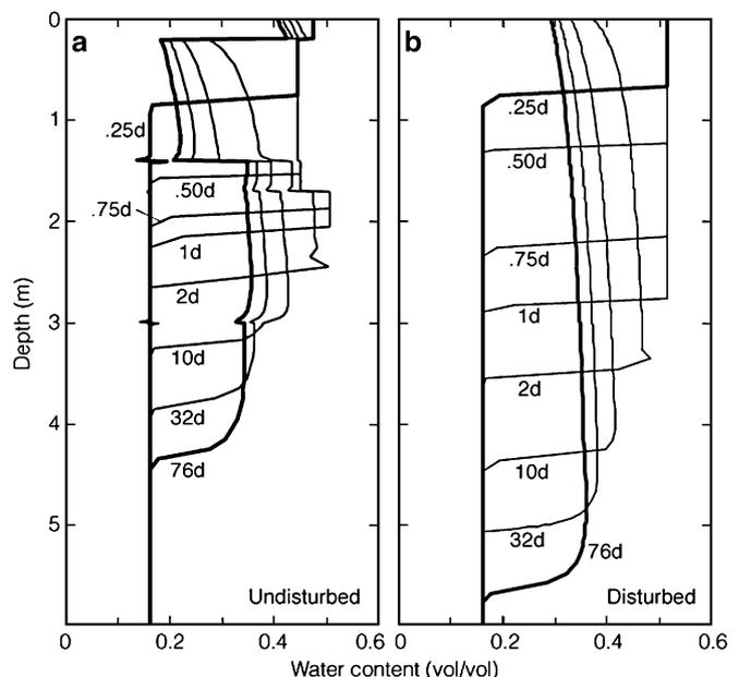
**Fig. 9** Infiltration and redistribution predicted by the basic one-dimensional model for **a** undisturbed and **b** disturbed soil at selected times
