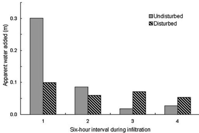
**Fig. 8** Water added during each of the four 6-h intervals of the 24-h infiltration period, computed from the measured water content profiles
