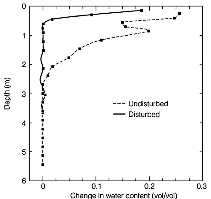
**Fig. 12** Measured change in field water content during the first 3 h of infiltration. This quantity may serve as an index of the hydraulic effect of preferential paths as a function of depth
