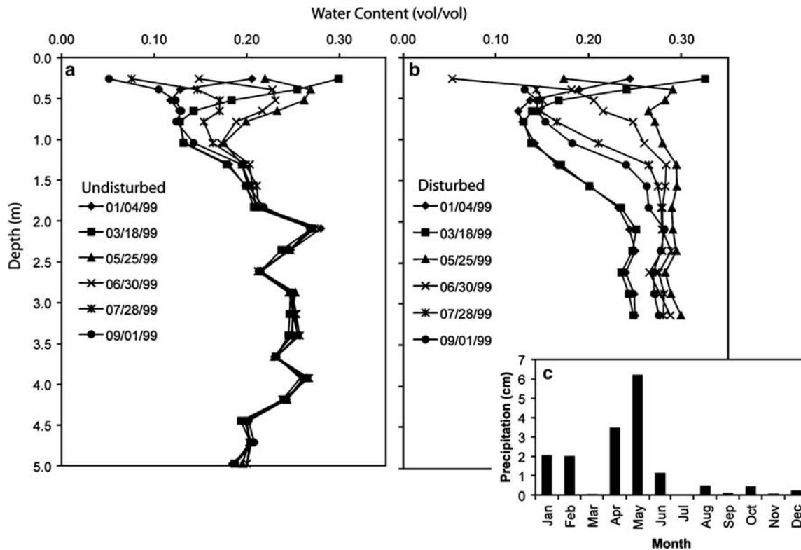
**Fig. 13** Water-content profiles measured in 1999 at neutron access holes **a** 2 and **b** 19. The artificial infiltration experiments had ended several years earlier, so these data show the response to natural rainfall and snowmelt, shown on **c**
