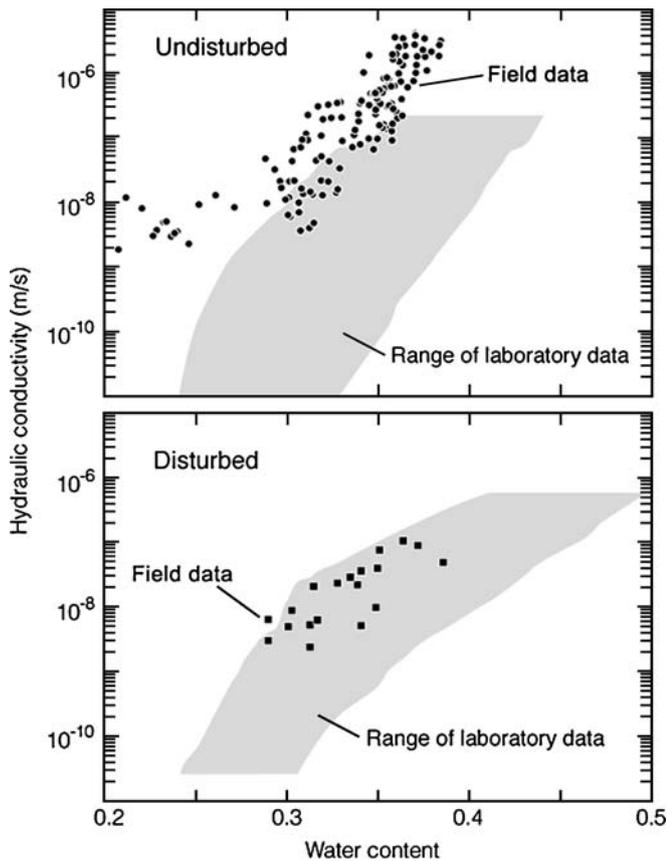
**Fig. 5** Field measurements of unsaturated hydraulic conductivity for undisturbed and disturbed soil, shown as *point symbols*. *Gray shading* indicates the range of one-step-outflow-method laboratory measurements from approximately the same depths
