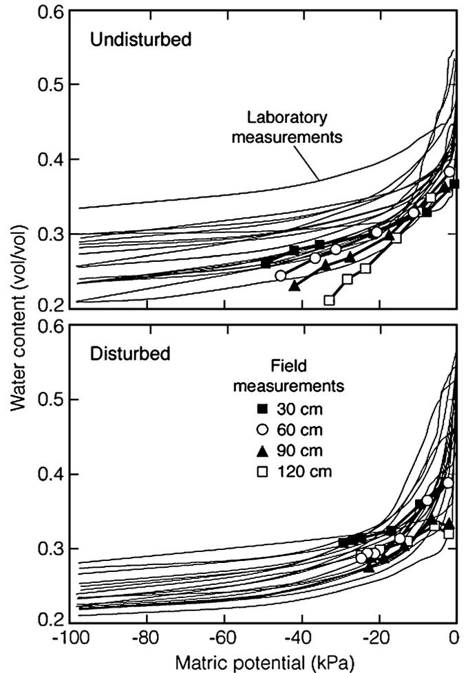
Fig. 4 Soil water retention curves measured by the SPOC (submersible pressure outflow cell) method and the field method for sediment samples in the undisturbed area and simulated waste trench. Only drying curves are shown. *Connected point symbols* show the field-measured data from the four tensiometer depths, and *curves without point symbols* show laboratory measurements on two replicate core samples at each of nine depths. Porosity appears as the endpoint of lab curves
