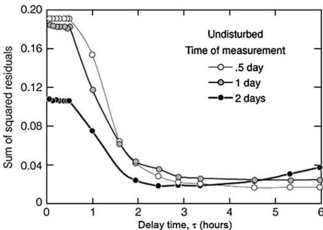
**Fig. 11** Goodness of fit to water content profiles measured 0.5, 1.0, and 2.0 d after the start of infiltration in undisturbed soil, as a function of the time  $\tau$  by which the initial condition was delayed in the simulation. Each of the three curves is based on 16 numerical simulations with different  $\tau$  values
