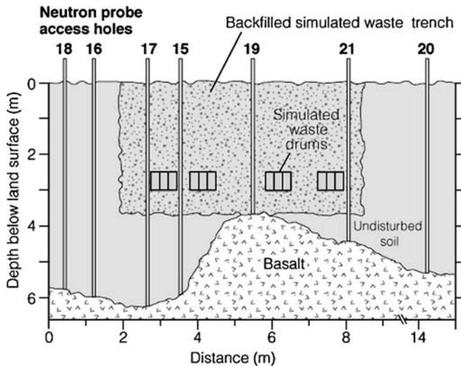
**Fig. 2** Cross-section of the simulated waste trench within the USGS test area. The number and location of waste drums is approximate. The shape of the soil-basalt interface is sketched on the basis of observations made during the construction of the simulated waste trench and the neutron access holes. Note that the horizontal distance scale is contracted between 9 and 14 m
